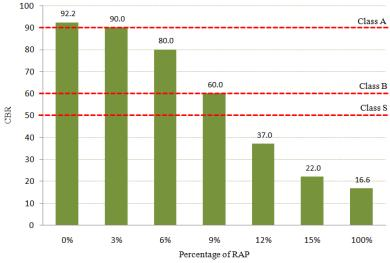
Figure 3. The Diagram of the CBR Values based on the RAP Percentage in Each Combination
