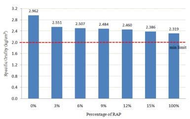
Figure 2. The Diagram of the Specific Gravity Values based on the RAP Percentage in Each Combination
